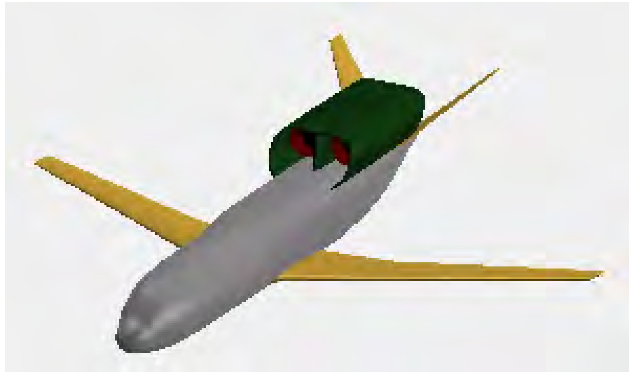
Figure 8.14: Configurazione EOF ( Engine Over Fuselage ), da [155].
