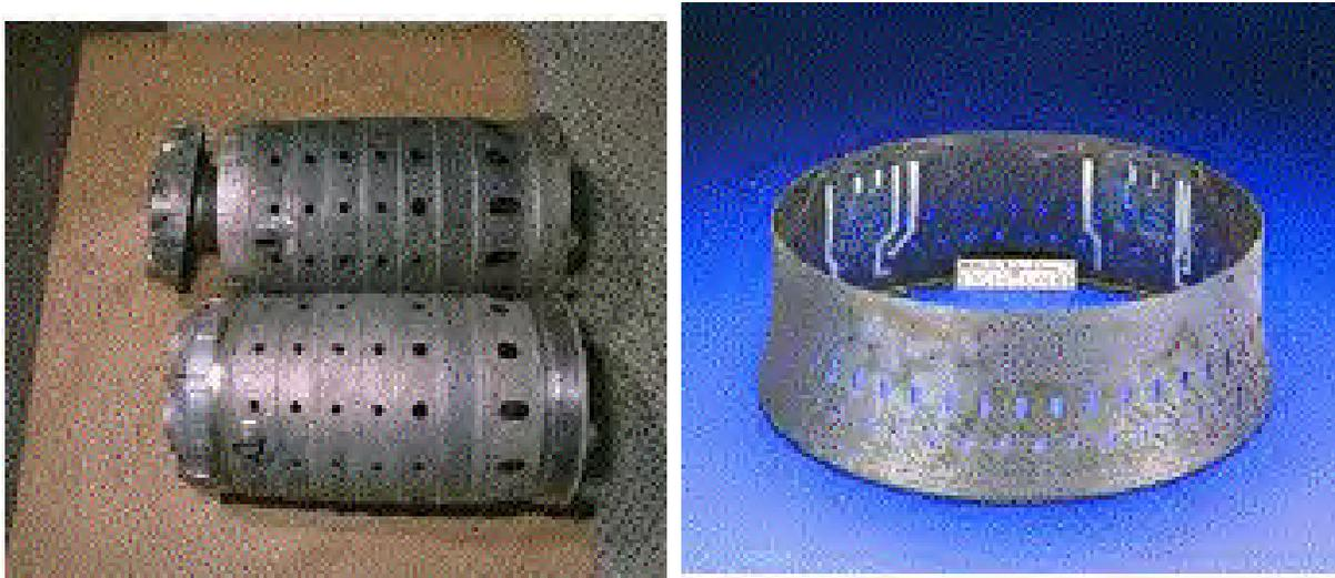
Figure 47: *Liners* of tubular (left) and annular (right) combustion chambers.
