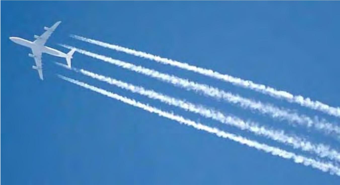
Figure 35: *Contrails* issuing from an aircraft.
