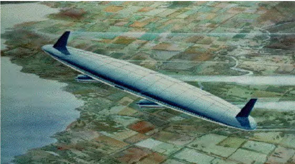
Figure 157: Oblique flying wing configuration.
