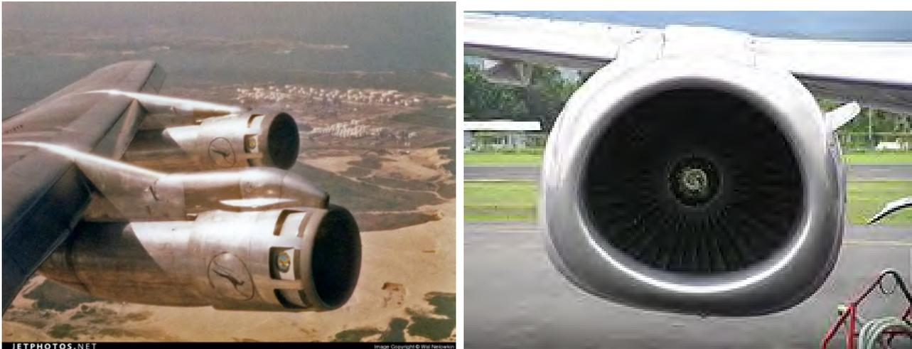
Figure 126: *Slats* (left) on the engines of a Boeing 707; (right) ‘hamsterized’ air intake of a Boeing 737 with CFM56 engines.
