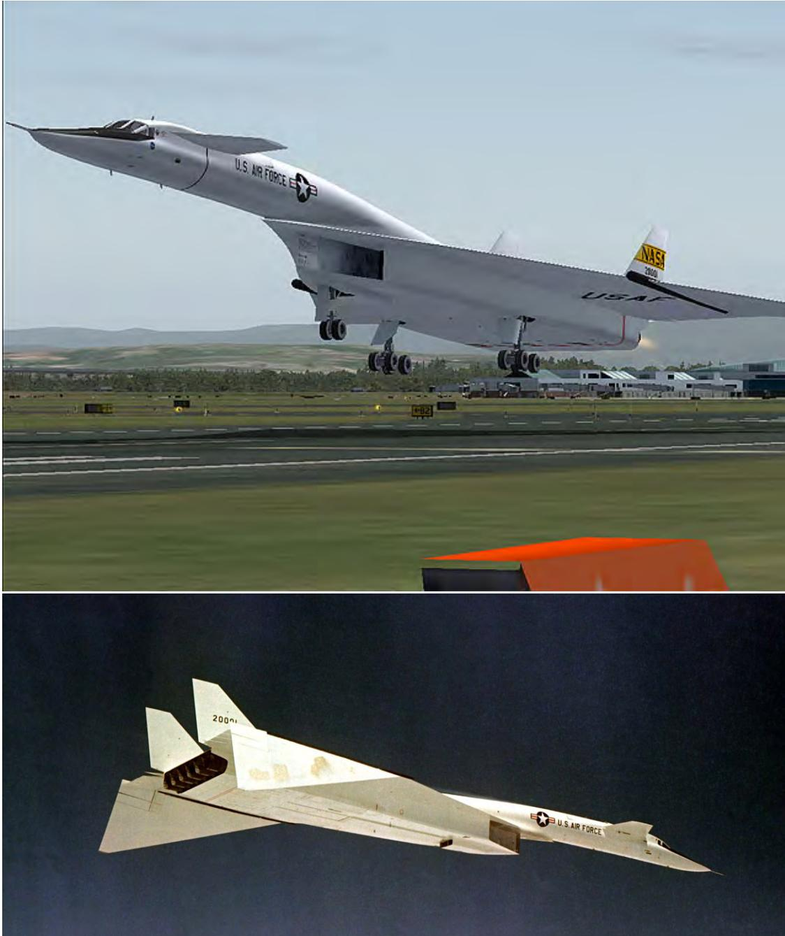
Figure 146: (top) XB-70 at take-off; (below) wing tips drooping at altitude.
