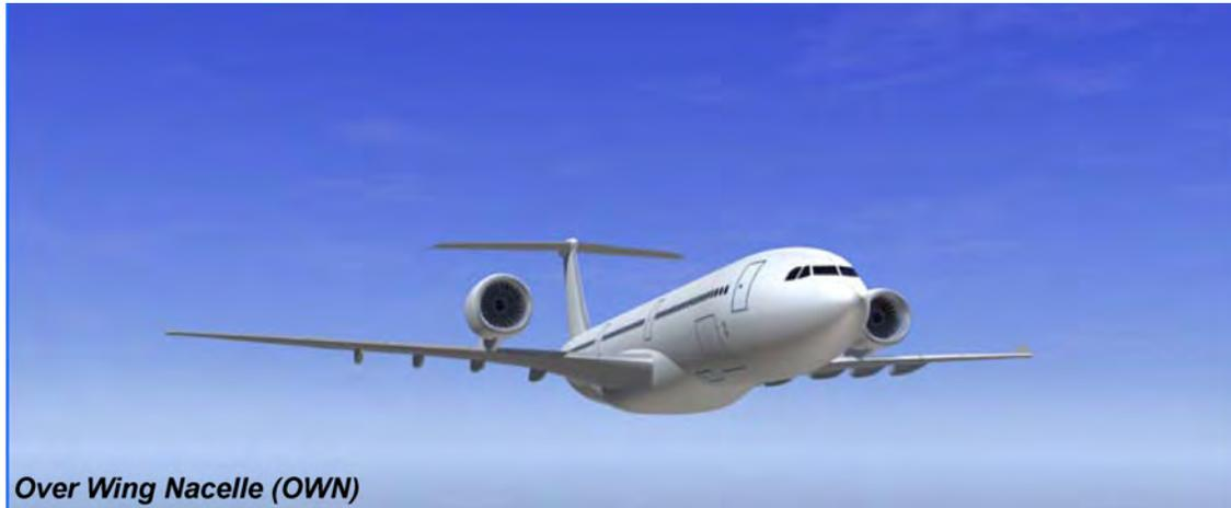
Figure 15: *Over the Wing Nacelle* configuration.
