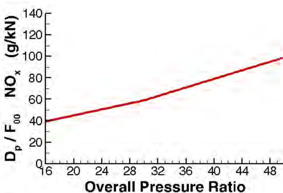
Figure 5: Limits on NO<sub>x</sub> emissions per LTO cycle *vs.* OPR.
