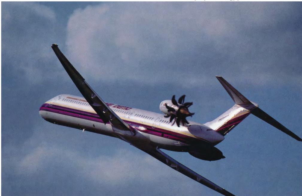
Figure 137: Propfan with contrarotating, pushing propellers.
