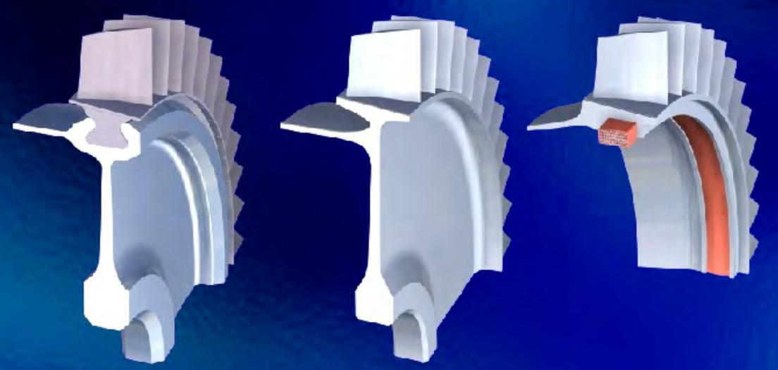
The image displays three cutaway views of compressor stages. The first shows a conventional design with a separate disk and blades. The second shows a blisk design where the disk and blades are integrated. The third shows a bling design, which is a blisk with a Ti MMC core, indicated by an orange layer.
