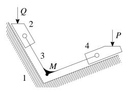
Given the (constant) velocity of the slider 2, evaluate the velocity and acceleration of point M attached to link 3.
