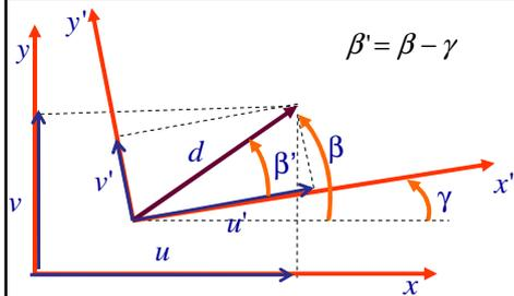
$$\begin{aligned} \cos \beta' &= \cos \beta \cos \gamma + \sin \beta \sin \gamma \\ \sin \beta' &= \sin \beta \cos \gamma - \cos \beta \sin \gamma \end{aligned}$$
