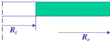
$$\begin{cases} 0 = B_1 + \frac{B_2}{R_i^2} - \frac{(3+\nu)}{8}\rho\omega^2 R_i^2 \\ 0 = B_1 + \frac{B_2}{R_e^2} - \frac{(3+\nu)}{8}\rho\omega^2 R_e^2 \end{cases}$$
